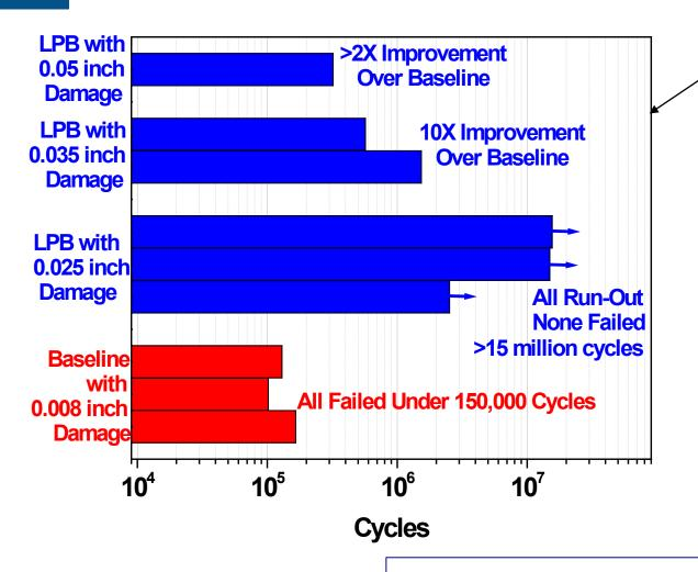
**Designed Compression Applied to GE 7F RO Blades for Erosion Mitigation**
