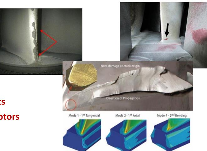
Erosion related damage tolerance requires frequent inspection, blending, and costly downtime.
